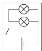
$$\frac{1}{R_T} = \frac{1}{R_1} + \frac{1}{R_2} + \dots + \frac{1}{R_n}$$
