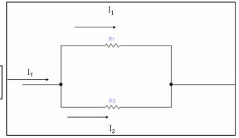
$$I_1 = \frac{R_2}{R_1 + R_2} I_T$$
